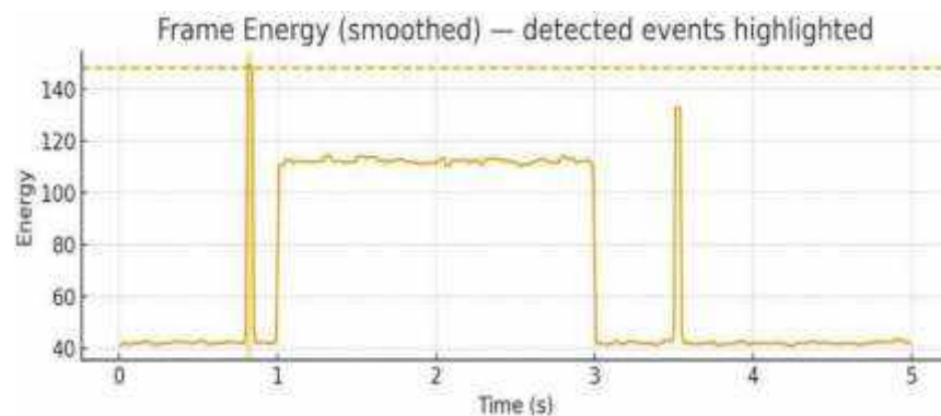
Figure: 1. G Smoothed Frame Energy Plot Showing Detected Acoustic Events
